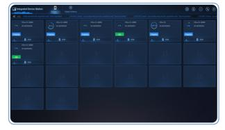
Running on the PC, IDS collects and stores digital evidence from the BWCs by multi-unit chargers. With intuitive GUI, you can review, manage, and share data simply and efficiently.
